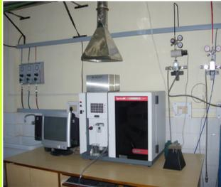
Atomic absorption spectrophotometer is available with the institute for the determination of trace elements in bio-environmental samples collected from mining and metalliferous industries.
